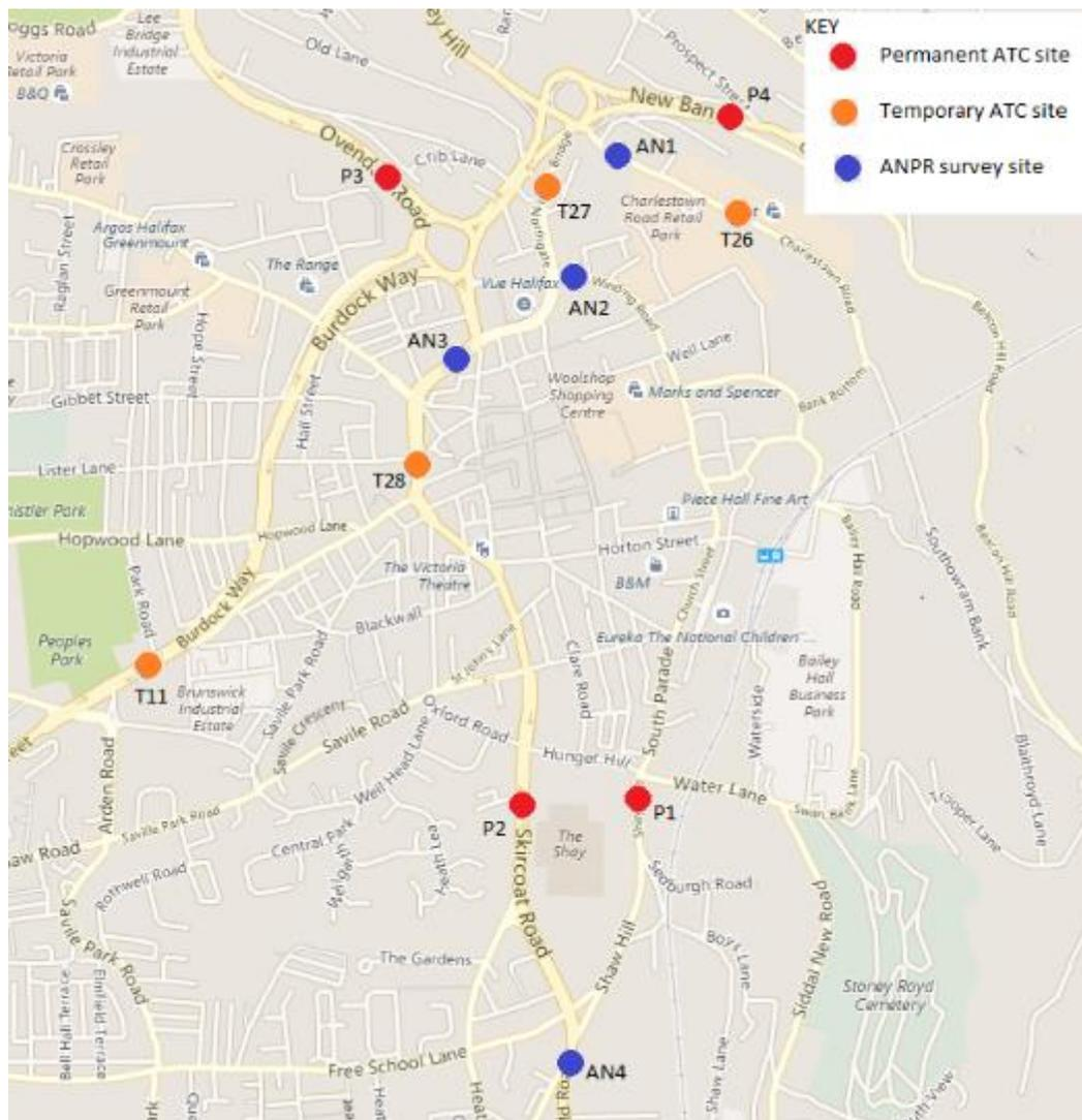
**Figure 6.1 – Automatic Traffic Counter (ATC) and Automatic Number Plate Recognition (ANPR) survey sites**
